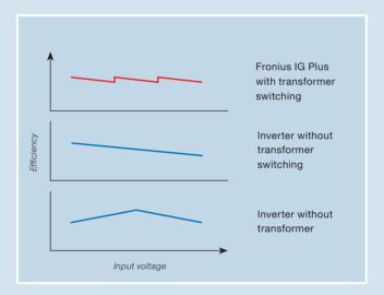
MIX™ Concept. Get the maximum power harvest out of partial load ranges, e.g. on cloudy days, through a clever combination of multiple power stages in each inverter. The power stages in Fronius inverters divide up the work depending on operating hours and only operate as many power stages as required to efficiently process available power from the PV array.
