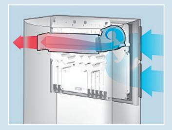
and the circuit boards while cooling the inverter components ensuring the inverter operates consistently. All circuit boards are also dipped in Conformal coating to provide an added measure of protection.
